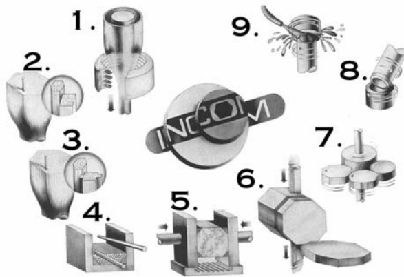
Figure 3– Incom, Inc. manufacturing process for fused fiber optic products, including fiber optic arrays.
